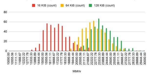
You can see how a single-stream with 16KiB send calls could often achieve the old maximum egress throttle of 16 Gbit/s, but would not hit the current maximum egress throttle of 32 Gbit/s. Using 64KiB or 128 KiB gets single-stream performance much closer to that. Add in a few more streams to hit the throttle.
