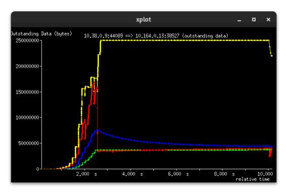
The vertical axis of this "owin" chart is bytes. The horizontal axis is time. The two lines of interest are the Yellow and the Red. The Yellow line is the receiver's advertised window. The Red line is how much data was outstanding on the connection at that time. The Blue and Green lines are simply different running averages of outstanding data.
